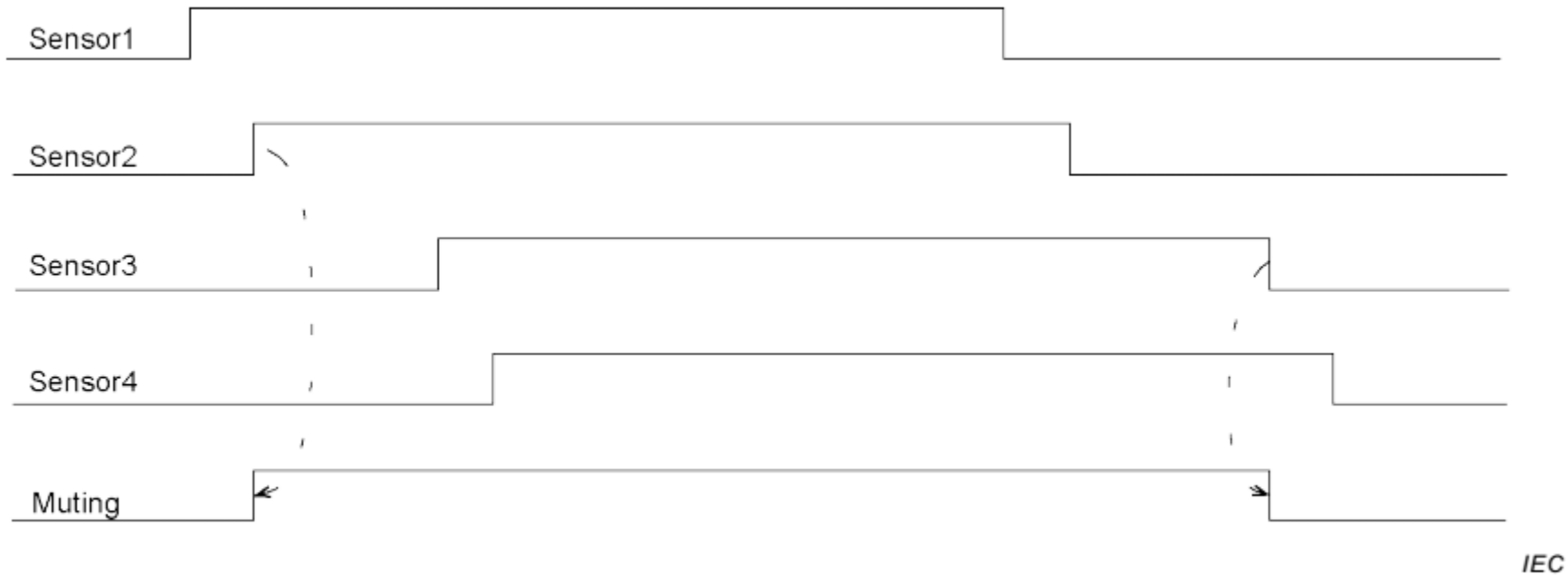
Figure D.9 – Timing diagram: four beams and sequence control
