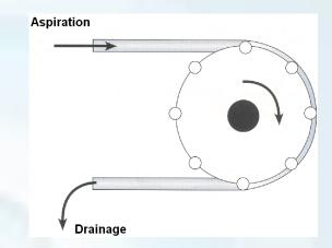
Vacuum can only occur in a peristaltic system when an occlusion at the tip (or a blockage in the line) occurs!
