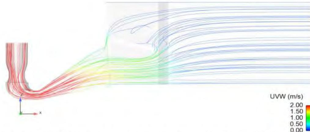
**Figure 6.** Side view of the flow pattern illustrated by streamlines colored by velocity magnitude; red color indicates velocity of 2 m/s or higher.
