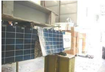
Failure of the strengthened beams with stirrups (side-bonding)
