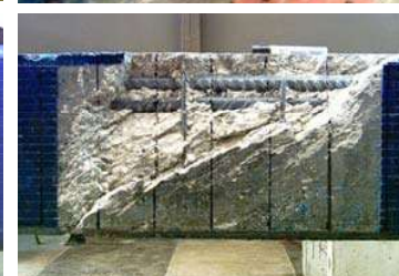
Failure of the strengthened beams with stirrups ("U"-jacketing)
