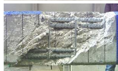
Failure of the strengthened beams with stirrups ("U"-jacketing)
