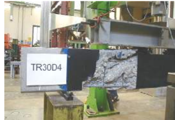
Failure of the strengthened beams with stirrups (side-bonding)
